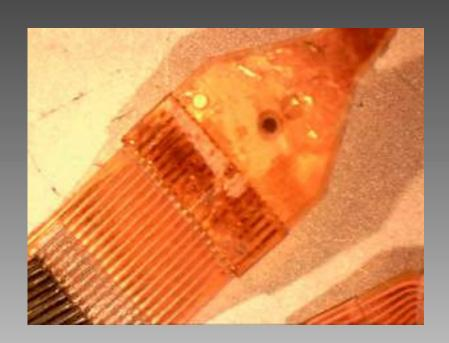
Micro flex cables soldering capability on 0.1mm leads
